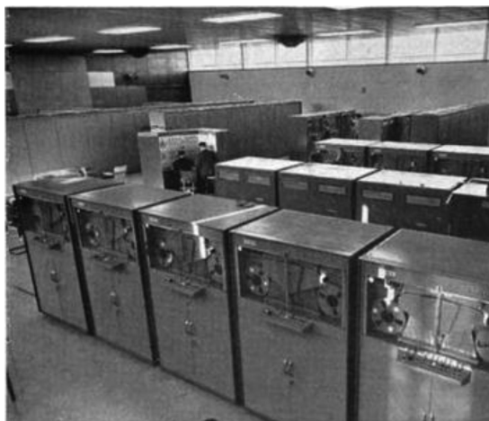
Figure 3. Photo of the EMIDEC 2400’s many tape drives for recording citizens’ pension account information, from the Report of the Ministry of Pensions and National Insurance for 1961, page 23.
