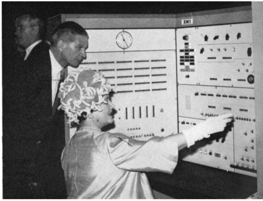
Figure 2. The Queen Mother inaugurates the EMIDEC 2400 at the Newcastle headquarters of the Ministry of Pensions, by pressing a switch that starts a “sort and merge” program. This particular program operated on over 200,000 items and took roughly 50 minutes to complete, according to the Ministry. (Photo from the Newcastle Chronicle and Journal , reproduced in the annual Report of the Ministry of Pensions and National Insurance for 1961, page 20.)
